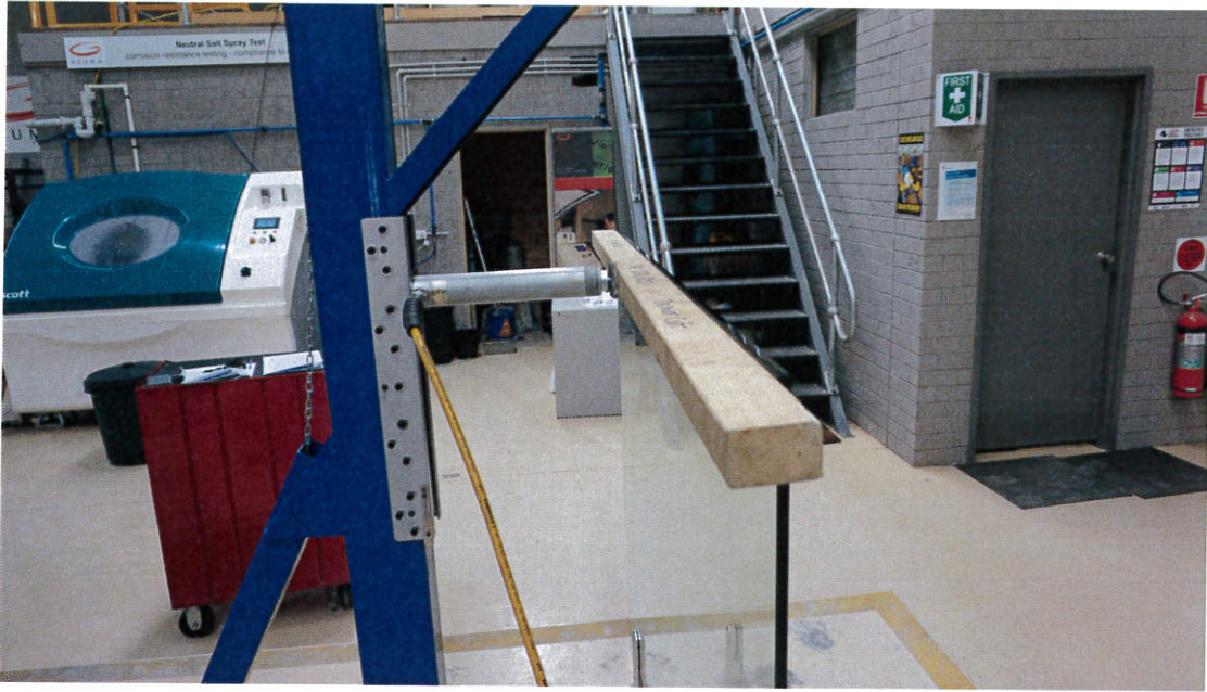
Figure 6: Horizontal Uniform Load - 350 N/m
