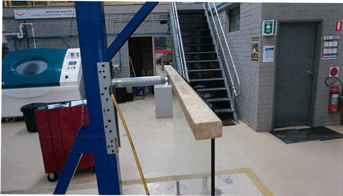
Figure 7: Horizontal Uniform Load - 750 N/m
