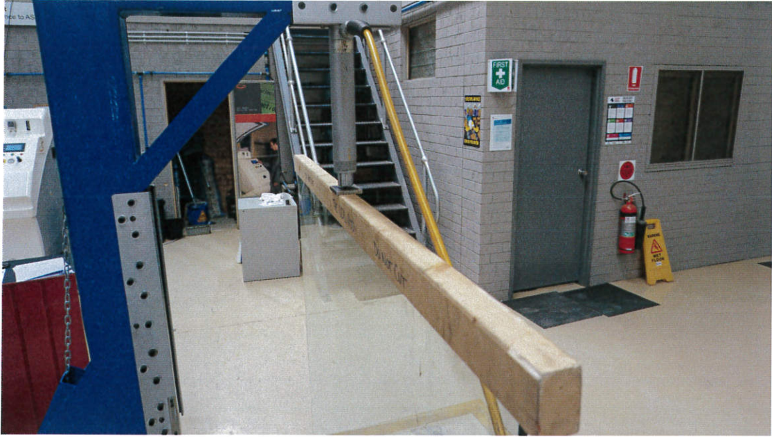
Figure 5: Vertical Uniform Distributed Load
