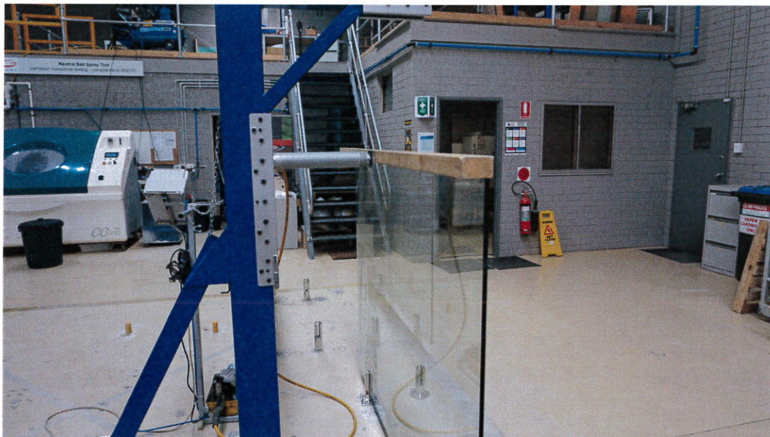
Figure 7: Horizontal Uniform Load - 750 N/m
