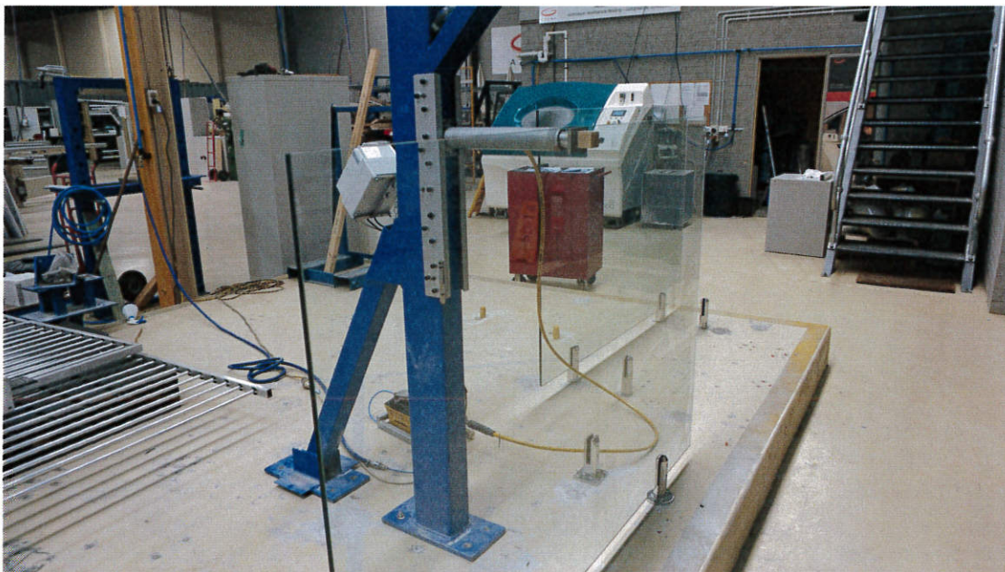
Figure 3: Outwards Push - Bend
