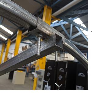
7) Now that the frame is complete, all bolts can be tightened, starting from the top of the tree.
