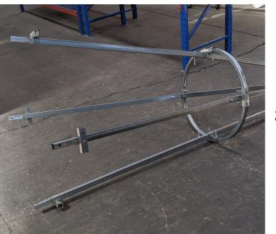
3) Join the middle frame bars to the upper frame bars.
